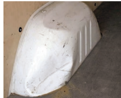
Deformation > 100 cm 2 am Radkasten
